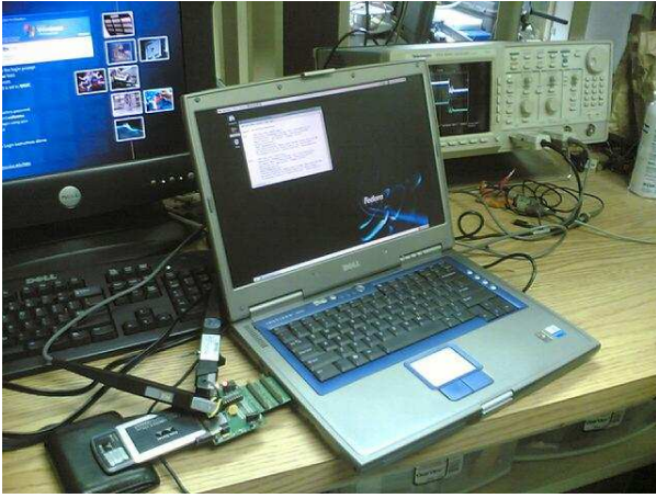
Fig. 1. Measurement setup used to determine energy characteristics of Aironet 350 wireless card in different modes.
