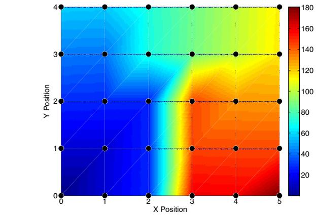
Fig. 10. SYNAPSE: snapshot of a single dissemination for a grid network of 30 nodes. Different colors represent different dissemination times (in seconds).
