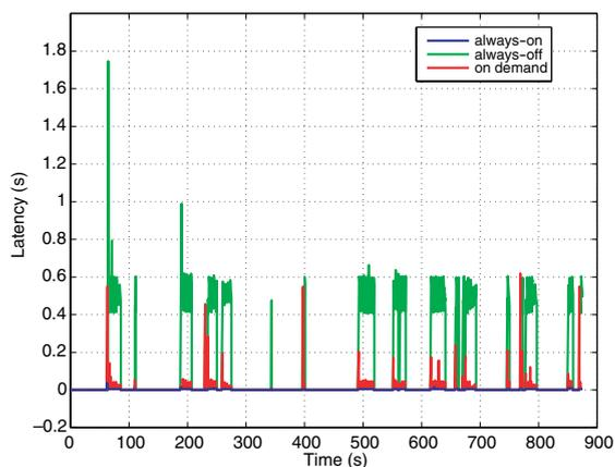
Fig. 10. End-to-end delay of one connection under on-off traffic, rate = 1 kbps.
