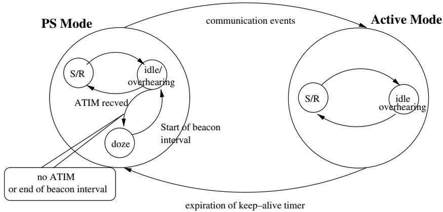
Fig. 3. State transition diagram for power management modes enhanced with IEEE 802.11 physical states.
