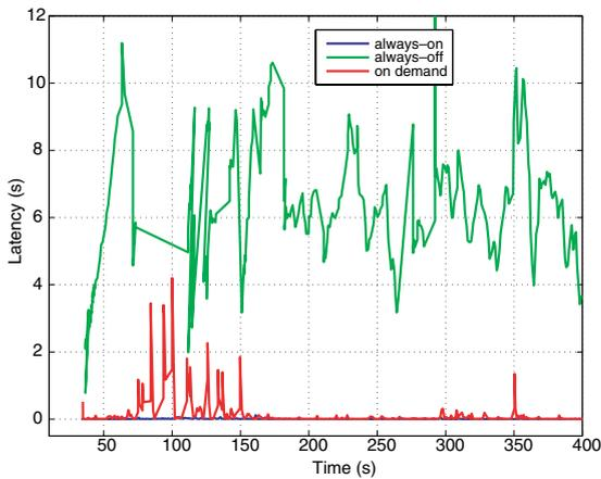
Fig. 13. End-to-end delay for one connection, speed = 20 m/s, pause = 50 s, rate = 1 kbps.
