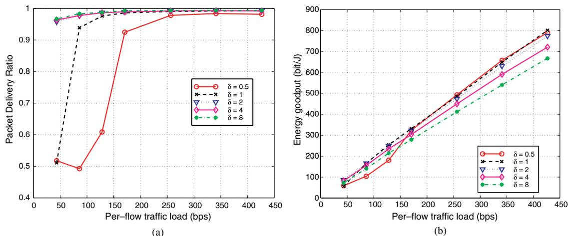
Fig. 6. Impact of different DATA\_KEEPALIVE timer, 30 on-off connections, on = 10 s, off = 100 s, 50 nodes, 1500 × 300 static network: (a) packet delivery ratio and (b) energy throughput.
