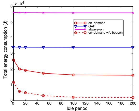
Fig. 15. Comparison with GAF, five on-off connections, on = 10 s, 85 nodes, 1000 m × 1000 m.
