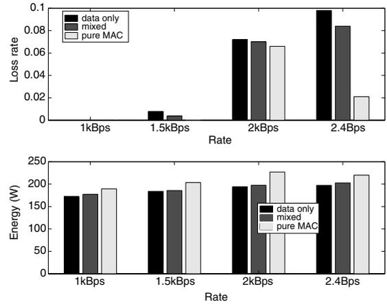
Fig. 5. Comparison of loss rate and energy consumption with and without cross-layer information.
