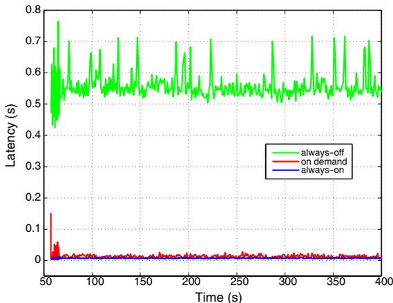
Fig. 8. End-to-end delay of one 3-hop connection, rate=1 kbps.
