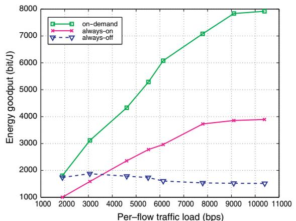
Fig. 14. Packet delivery ratio and energy goodput vs. traffic load. 10 long-lived CBR connections 50 nodes, 1500 × 300 static network.
