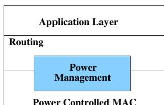
Fig. 2. Location in the protocol stack of our power management framework.
