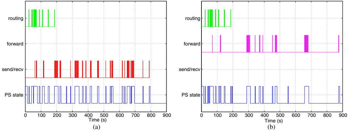
Fig. 11. Actual duty cycles of a node: (a) a data source and (b) a router node.
