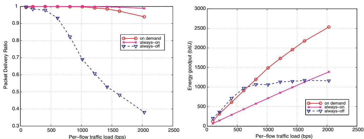
Fig. 9. Packet delivery ratio and energy goodput vs. traffic load. 30 on-off connections, on = 10 s, off = 100 s, 50 nodes,  $1500 \times 300$  static network.
